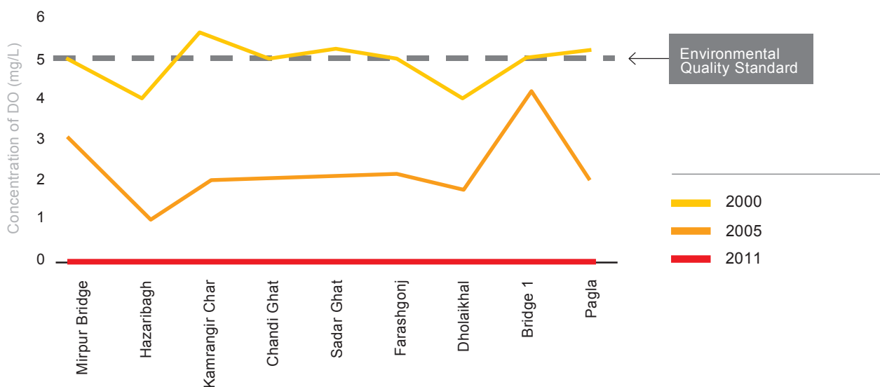
Figure 12: Comparison of the DO value changes in Buriganga at critical locations in January 2000, 2005 and 2011
